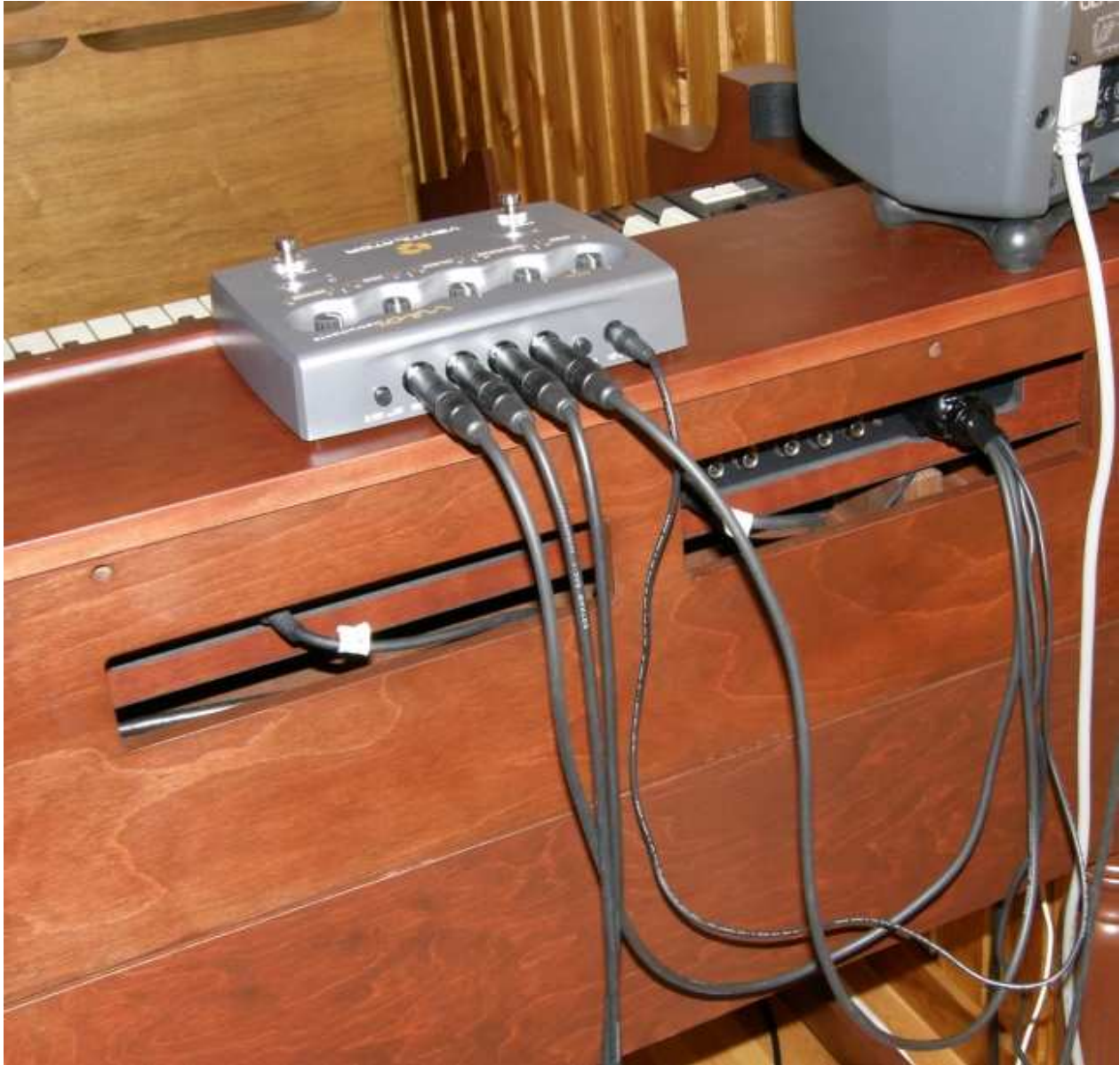
Fig. 4) Picture of the adapter cable in use connected between XK-3 and Ventilator
